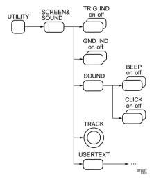
Toggle softkey to display trigger level indication.
