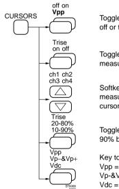
Toggle function softkey to switch cursors on and CURSORS off or to select the Vpp mode.
