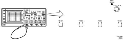
Figure 3.9 Direct trigger setup
