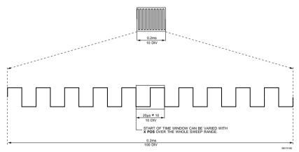
Function of timebase magnifier and X POS control
