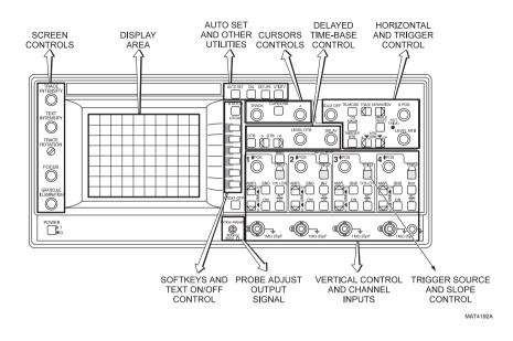
The controls on the front are grouped by function. In this chapter, a description for each group of controls is given in the following sequence:
