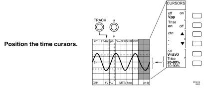
The risetime is now displayed in the top line on the screen as 'Tr=...ms'. When ' $\Delta$ V' is selected, ' $\Delta$ V=...V 20-80% is displayed at the same time. When 'V1 & V2' is selected, 'V=-.../+...V' is displayed.
