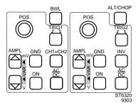
The CH1 and CH2 section of the PM3084 is shown on the left. Refer to section 4.1 for the differences between model numbers PM3082/PM3084.
