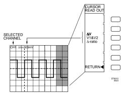
$\Delta V$  is the voltage difference between the voltage cursors (readout:  $\Delta V$ =...V).
