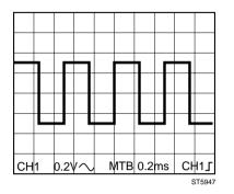
Step 4 Check the pulse response before doing any measurement. If the pulse shows overshoot or undershoot, you can correct this by using the trimmer in the probe's body. This prevents measurement errors! Chapter 4 describes how to adjust the pulse response.
