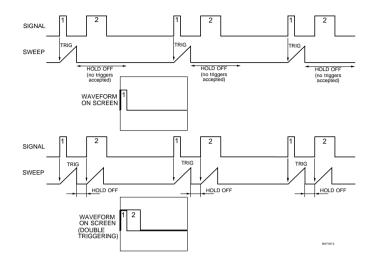
Using HOLD OFF to suppress double triggering
