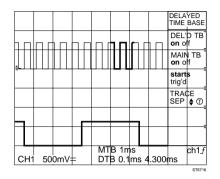
Figure 3.15 The main timebase trace and the delayed timebase trace displayed simultaneously
