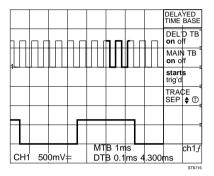
The main timebase trace and delayed timebase trace are displayed simultaneously.
