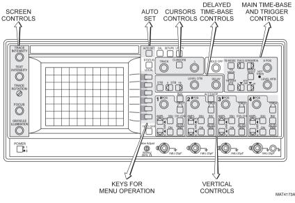
Figure 3.3 Front-panel layout PM3094
