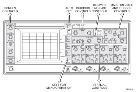
Figure 3.4 Front-panel layout PM3084
