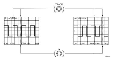
At the top of the screen, the time distance between ( $\Delta T$ ) is displayed. This is used for timing measurements.
