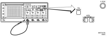
Figure 3.8 Timebase setup
